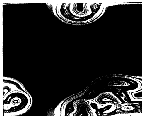
FIG. 5. Island formation on a uniformly oscillating Pt(110) surface. The values of the external parameters p_{CO_e}=3.992 \cdot 10^{-5} Torr, p_{O_2}=1.17 \cdot 10^{-4} Torr, T=545 K correspond to relaxation oscillations of the integral reaction rate. The other parameter values are D_i=0 , V_{ML}=0.225 l/ML, and J=360 l/s.
